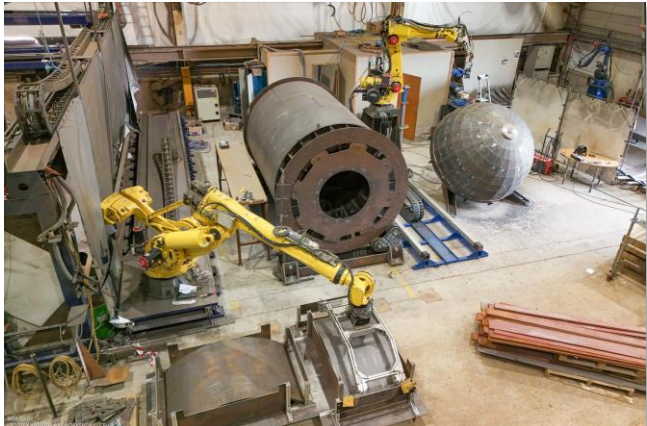
Installed Production Cell and tank sections partially complete
