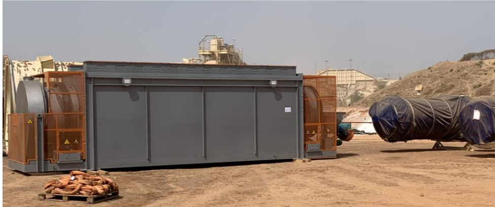
Package 2/3: Acid wash and elution columns and carbon regeneration kiln
