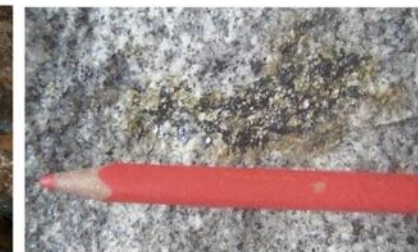
(d) Typical freshly broken faces in the monzodiorite containing disseminated chalcopyrite and pyrite.
