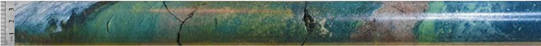
Semi-massive sulphide mineralised skarn with visual chalcopyrite-pyrite-magnetite on the contact of a feldspar porphyry apophysis (right) in limestone (left) at 58.30-58.62m 1 .
