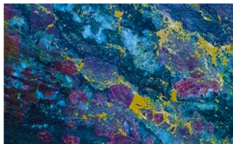
Photo of Chalcopyrite-Quartz-Garnet-Amphibole Breccia 1 polished rock chip grading 11.9% Copper from the Wolf Mountain area showing similar mineralisation and alteration styles to core above.
