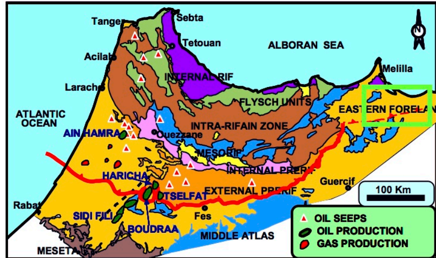
Figure 1: Simplified geological map of northern Morocco showing oil seeps and production with the location of Beni Znassen basin.
